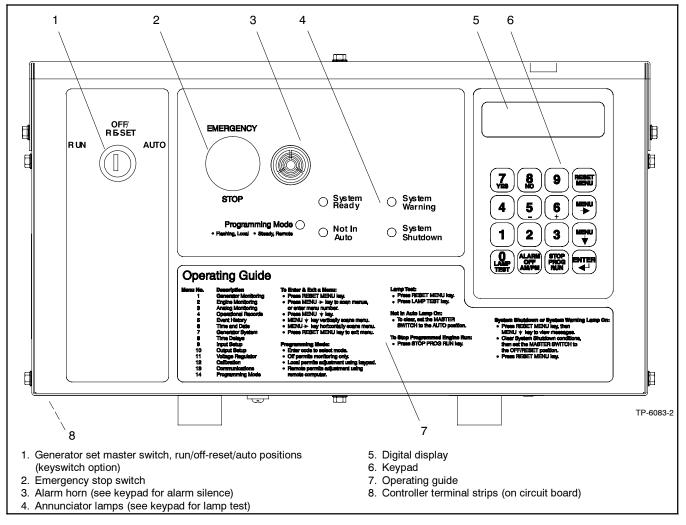
Figure 1-2 550 Controller with Keyswitch Option
